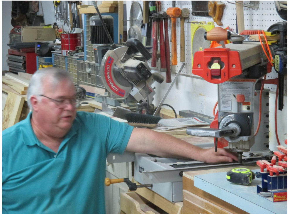
Brian Harrell demonstrates the alignment of a radial arm saw.
