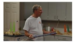
Bob Busfield shows how to wrap dowels with painter's tape prior to cutting on a band saw or miter saw to avoid flying pieces.
