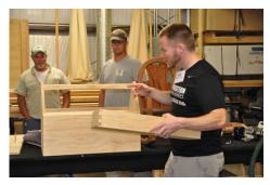
Matthew Mohon built a tool box with dovetail joinery. He used a dovetail jig with magnets that keep the saw close to the marked line. He used a Lie-Nielsen router plane to cut the rabbets.
