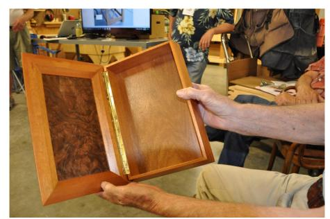
Tom Gustafson built a birch box inset with walnut burl following an article in Fine Woodworking. The spline grooves are cut while the box is still rectangular; after the splines are inserted, the sides are beveled.
