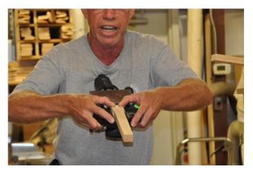
Jeff Horchoff shows how he uses a Festool Domino to make the top bar and sides for the top bar hive. The entrance to a hive can be very small, e.g., a one-inch diameter hole or a two inch by one-half inch slot. The small opening makes it easier for the bees to defend their home.
