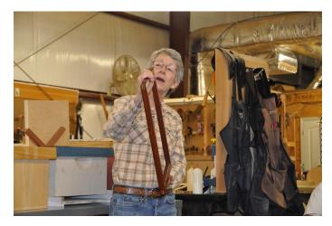
Pat Robbert made a picture frame out of sapelle with maple miter keys. The simple jig she used for cutting the miter slots is clamped to a crosscut sled.
