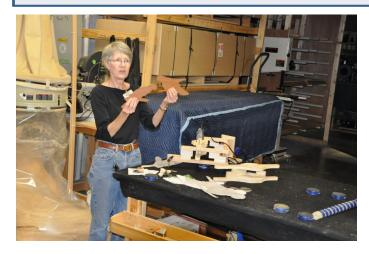
Pat Robbert built a 3-D pantograph from plans by Matthias Wandel (www.woodgears.ca). She used the stylus to trace an enlarged template made of matte board while the Dremel cut the design out of sapelle.
