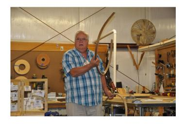
Brian Harrell does some steam bending with kiln dried ash. He first soaked the wood for five days in a seven-foot long 2" PVC tube filled with water and fabric softener. He made a drying frame from an 84" long piece of 1.25" wide 16 or 18 gauge steel strapping.
