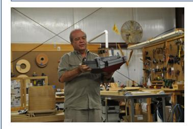
Bill Pecoul shows a remote control tug boat he built using a web available design called the Springer. His is all wood and must weigh 8.5 lb or more, have a 4 sq. in. rudder and a 2" three blade propellor for competition.
