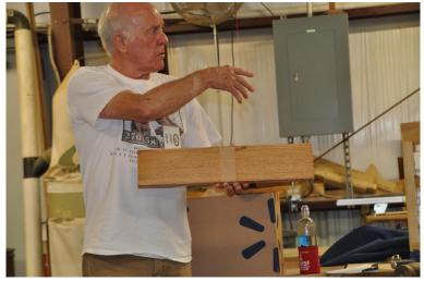
In this test, Henry Simon filled the grain on one side of the board by creating a slurry using 400 grit sandpaper and linseed oil. When dry, he sanded both sides and applied a wipe-on oil finish. The filled side feels slightly smoother.
