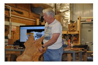
Randy Turner resawed a thick slab of old cypress to make a commemorative plaque for his grandson's Eagle Scout Troop. To do the resawing, he strapped a chain saw to the table saw table with the blade parallel to the table and fed the slab into the 12 inch blade from all sides. Small cracks were filled with super glue and wide cracks with Gorilla glue. He carved the scout symbol with a hand-held router.
