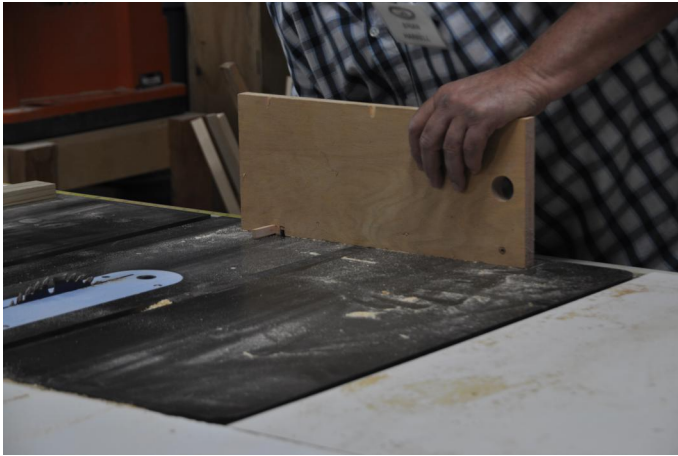
The finger joint jig is attached to the miter gauge.
