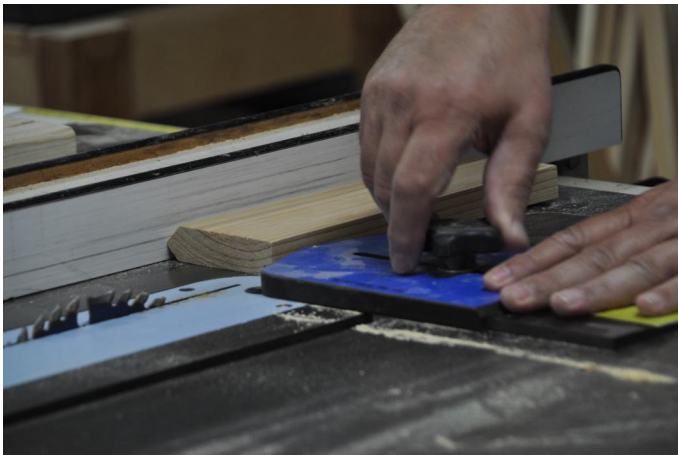
The finger joint jig is attached to the miter gauge.
