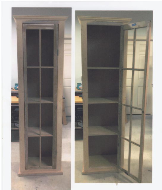
Jack Terry built these cabinets using Kreg pocket screws with their holes on the outside of the cabinet. He prepared moulding with a Woodline router bit and used it to cover the pocket holes. He noted that the Kreg pocket hole system has a new HG size socket with a 1/2" drill bit and larger Kreg screws that have the strength to join 2x4 assemblies.
