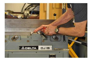
Henry explained that the jointer is the most important tool in his shop. He uses it to get one flat side and then one edge square to the side. Watch the grain of wood to avoid tear out. If the wood is cupped, place it on the table concave side down. Use a push stick. Always have the safety guard in place.
