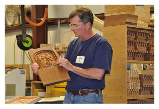
Al Gahn shows a carving for Stations of the Cross at the Abbey. The CNC machine spent 6 hours to make it, using a 1/32" ball nose bit. The plaque made from mahogany was successful, but the lighter wood, below, did not route cleanly. He gets the CNC programs online. The software with his machine allows him to enlarge or reduce the patterns, but not edit them in any other way.
