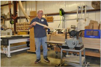
Joe uses the planer after the jointer has made one side of the wood flat. Snipe, a gouge near either end, can occur because of the pressure from the infeed and outfeed rollers on a planer. Some strategies to avoid snipe are to use a board that is longer than you need, to precede and follow your board with a similar board, to hold the trailing end of the board up at the entrance and to hold the leading end of the board up at the exit, and to cut with the grain.
