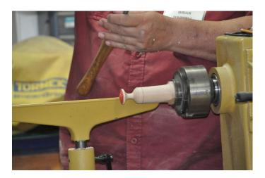
Finally, Brian uses a skew tool to cut off the completed finger spinning top from the blank.
