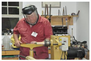
Next, Brian shapes a gentle point on the end of the wood blank. He then uses a spiral tool to make spiral designs on the end. In the third picture, he is coloring the spiral design using a red Crayola Marks-a-Lot.
