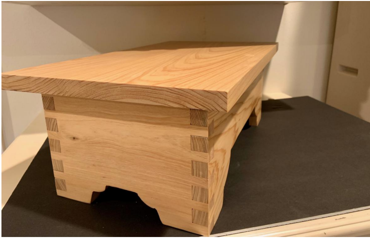
Jack Terry built this foot stool using the Leigh D-4 Dovetail jig.
