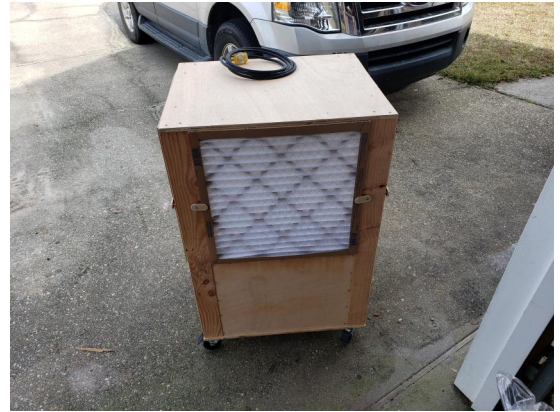
Last month, Aaron Mahnke told us about his air filtration unit. Here, you can see how he built the unit from a 220 V squirrel-cage furnace fan. The enclosure has pleated filters on four sides. He said there is a YouTube video showing how to make it on the Jay Bates channel, air filter for shop.
