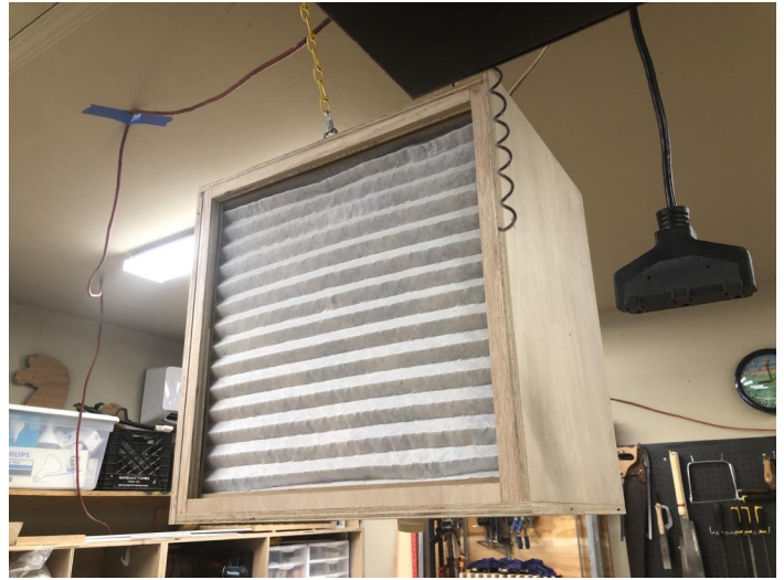
Jonathan Crowder built an air filter for his shop using two fans, a box, and three 20x20x1 inch filters.
