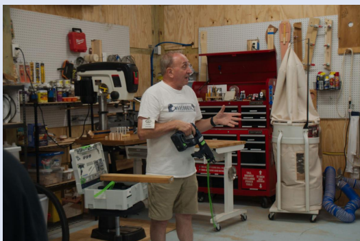
Clark Gristina enjoys the quality of Festool products. This drywall gun is a prime example. It accurately places screws into drywall and can also be used on studs. When available, a reconditioned product is discounted 25%.
