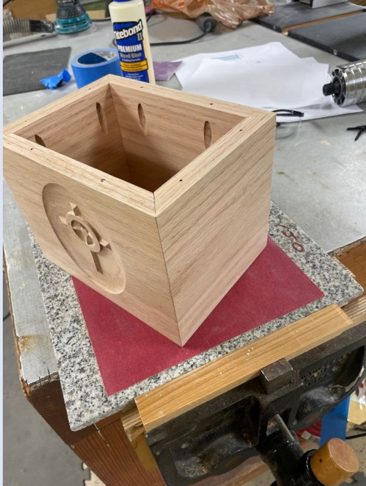
Here is the urn, 1 cu-in per lb, before the top is attached.
