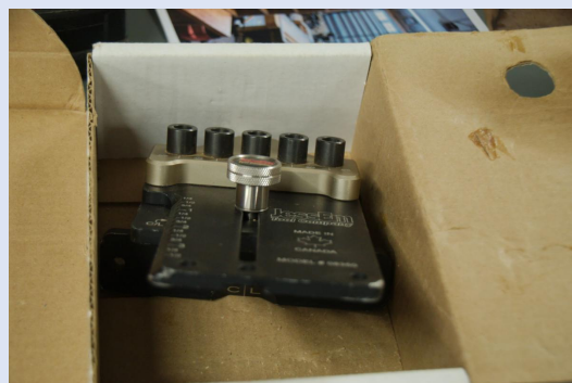
The jig comes with a registration pin and three sets of bushings for the
