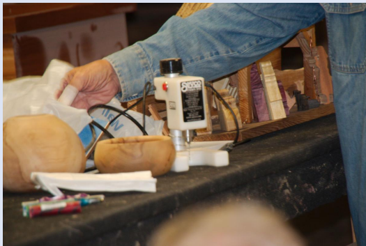
Craig shows a Seyco Scrollers Drill Press which uses drill bits sized from #50 to #80.
