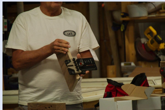
The jig has an adjustable fence with a 1/4" to 3 1/2" reach and indexed adjustment in 1/8" increments.
