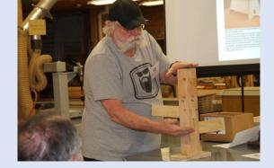
Bob Busfield showed an INSIDE wood ruler - the measurements that start with 1 are on the inside. Most wood rulers are OUTSIDE rulers with 1 on the outside. The bulk of the ruler can be in the way of a measurement with the outside ruler.
