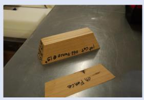
Ron Walker brought in a flared-sided box that he uses to layout dovetails with compound angles. This is similar to Roy Underhill's tool tote. One can use an online calculator for mitered and butt joints, but another tact is to set the table saw blade to the slant angle of 19 degrees, make a few specific cuts on a block of wood, and this will yield a jig for setting the table saw to the correct compound angle for the butt joint. **Chad Stanton** has a YouTube video that explains the process.
