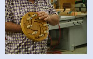
Warren also showed a Longworth chuck that is used on a lathe to hold a bowl for signature work. A guild in Australia patented the design after Longworth's death and gave the proceeds to his widow.
