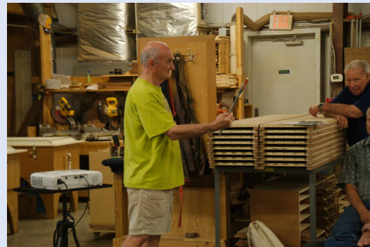
Joe Perret demonstrates the use of ammonia to restore a plastic tool handle.
