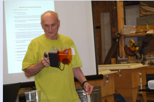
Joe Perret shows a LaserPecker portable laser engraver that he programs on the computer.
