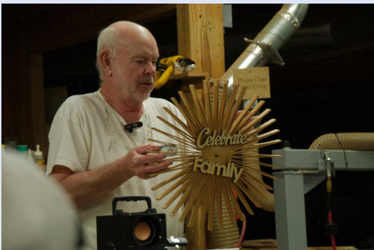
Tom Gustafson describes how he cut this wall art from a 3/4" x 6" x 8" piece of wood. He cut with the grain from alternating sides at the bandsaw.
