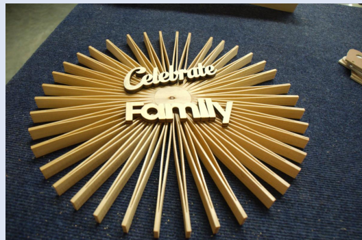
Tom Gustafson describes how he cut this wall art from a 3/4" x 6" x 8" piece of wood. He cut with the grain from alternating sides at the bandsaw.
