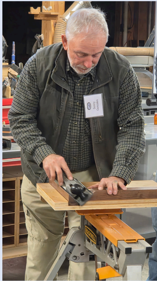
Here Sonny uses a shooting board that includes a vertical 45 degree angle.
