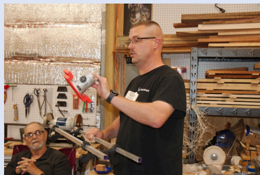
Aaron Mahnke shows a slab flattening jig he uses to flatten the top of a breadboard or wood slab.
