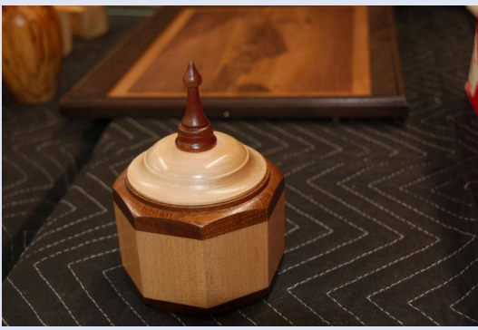
This pot uses miter joints to connect the pieces cut using his polygon cutting jig.
