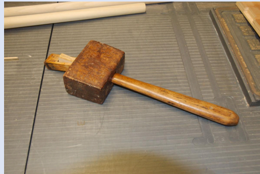
Ron's mallet, dated 1899, has a sliding dovetail joint in it.
