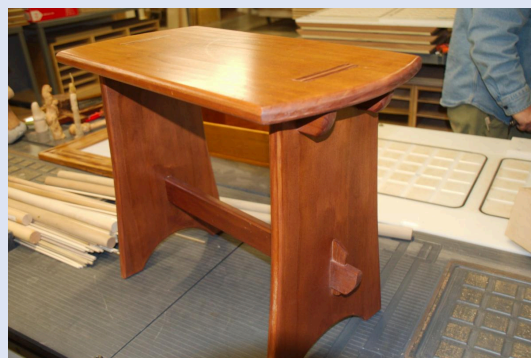
John Fisher shows the locking miter joint.
